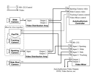
Figure 1. Schematic diagram of a typical AutoAuditorium System
