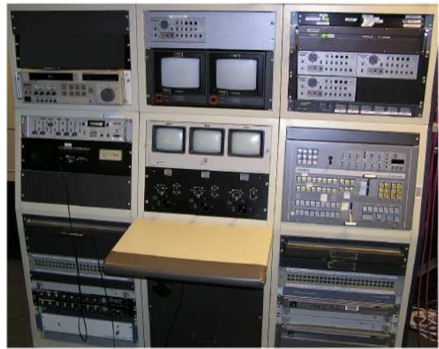
Figure 1: The Distributed Auditorium Console. Notice the three camera monitors, each above a cluster of controls for that camera.
